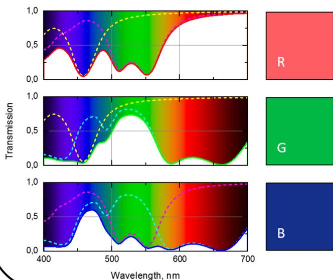
Fig. 3. RGB functions (solid lines) can be computationally derived from other color functions like CMY functions (dashed lines) found by similar parameter sweeps of Silicon nanodisk dimensions. Color representation (right) is shown according in CIE 1931 standard. The levels of RGB reach 90%, 70% and 60% respectively. Similar results can be obtained if the CMY filters would be used in a two layer system.
