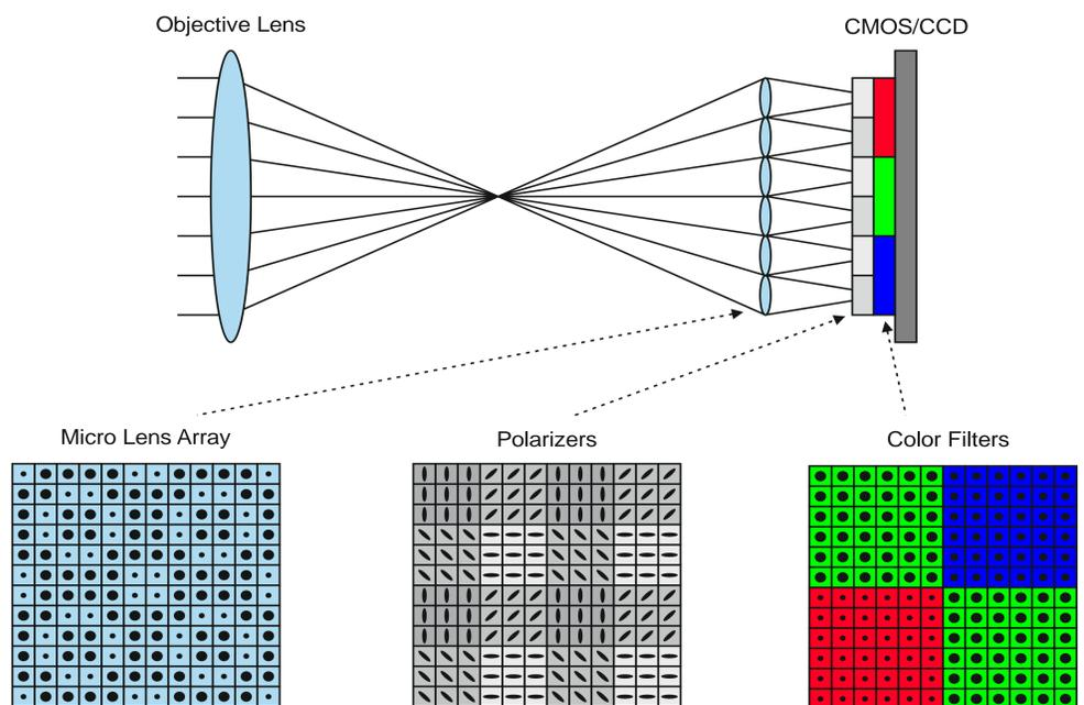
Fig. 1. Schematic representation of plenoptic camera using metasurface elements.
