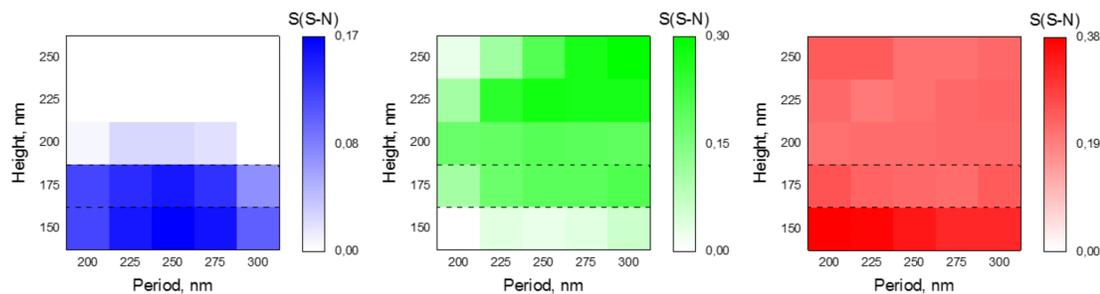
Fig. 2. Parameter sweeps of Silicon nanodisk for the best RGB filter function. At each period-height configuration full diameter sweep takes place until the best signal is found. The dashed lines highlight the constant height at all ranges for optimal manufacturing.
