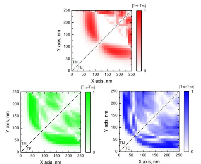
Fig. 5. Polarization sensitivity  $|TE-TM|$  dependence on the dimensions of Silicon ellipsis at RGB. The TE and TM polarization are aligned along X axis and Y axis, respectively.
