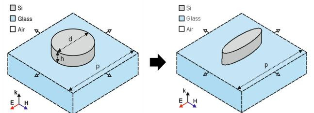
Fig. 4. Transformation from nanodisk to polarization dependent structure.
